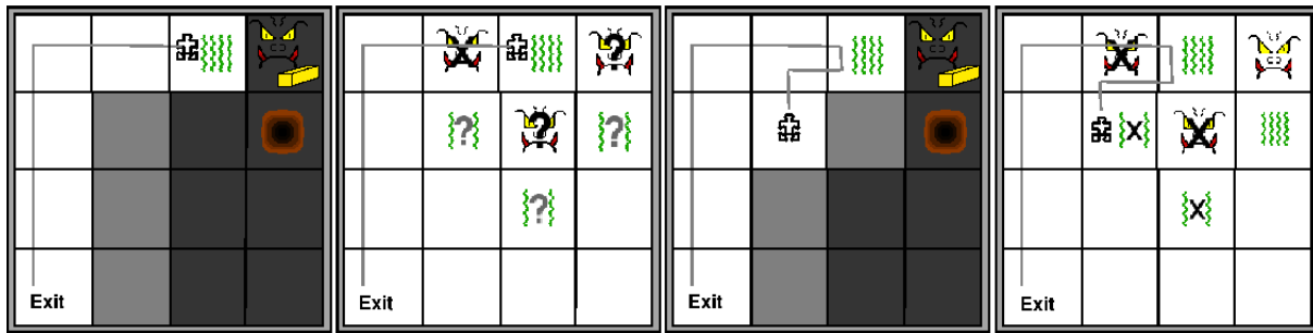
Figure 4. Four maps representing two situations in the Wumpus World. The first and the third maps show what the agent already knows about the environment: white squares represent visited positions; black squares represent not visited positions; and grey squares represent not visited positions which were inferred to be safe. The second map shows the agent's hypothetical reasoning about the first map, and the fourth map shows the same about the third map. Squares labelled with “?” denote hypothesis; squares labelled with “X” denote a false hypothesis.
